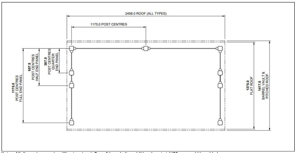
Note – All dimensions are in millimetres (mm), For a 3 bay shelter additional post at 1175mm would be added.
