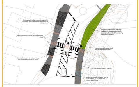
Extensive tree and ecological surveys have been undertaken and the route designed so that very few trees will be affected. The construction of the path through the trees is of a no-dig permeable type, which will minimise any impact on the tree roots.
