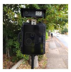
The valuable data acquired by the SID enables the efficient deployment of the ASWC in locations known to be problematic in terms of vehicles exceeding the speed limit with the consequent transfer of the data of offending vehicles to the police for further action. With these two machines operating in tandem, we are set to tackle speeding in the parish much more effectively.
